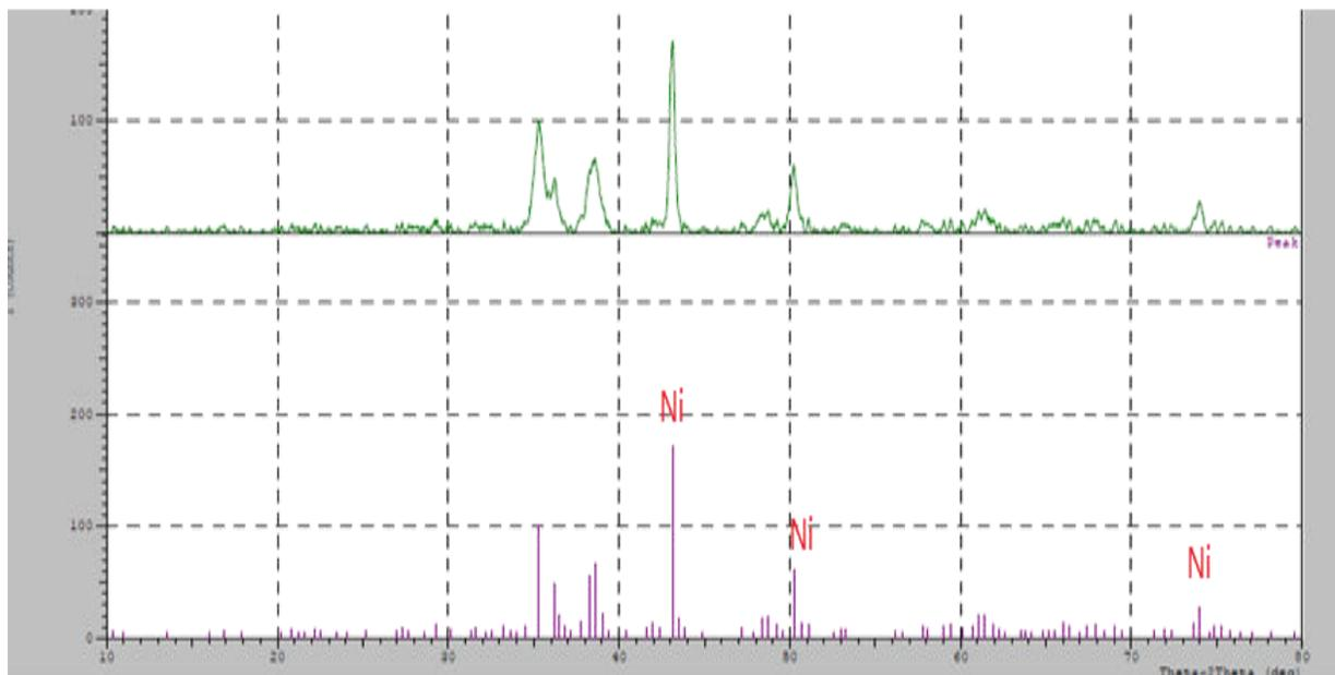
**Fig. 3: XRD patterns of bio-synthesized Ni NPs sample**
