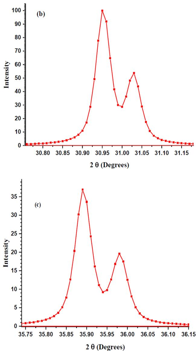
Fig. 3: (a) XRD spectrum of silicon hydride (b) enlarged prominent peak-1 and (c) enlarged prominent peak-2 of silicon hydride nano-cluster.
