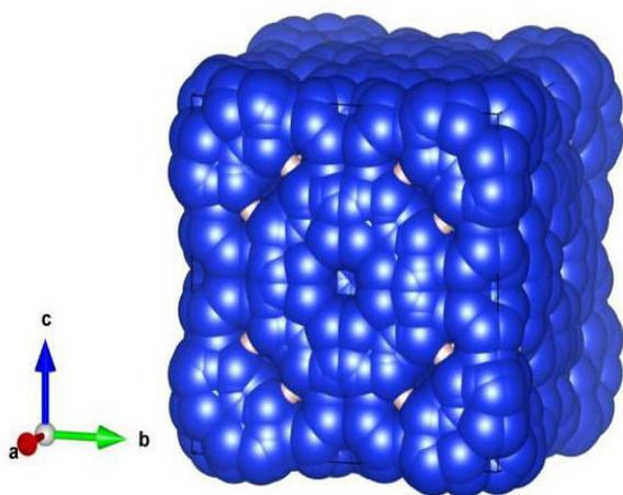
**Fig. 2: Unit cell of silicon hydride of dimension 5Å**
