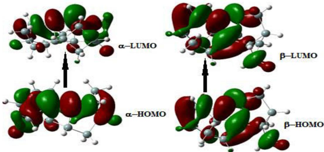
**Fig. 9: First HOMO-LUMO orbitals of silicon hydride nanocluster**
