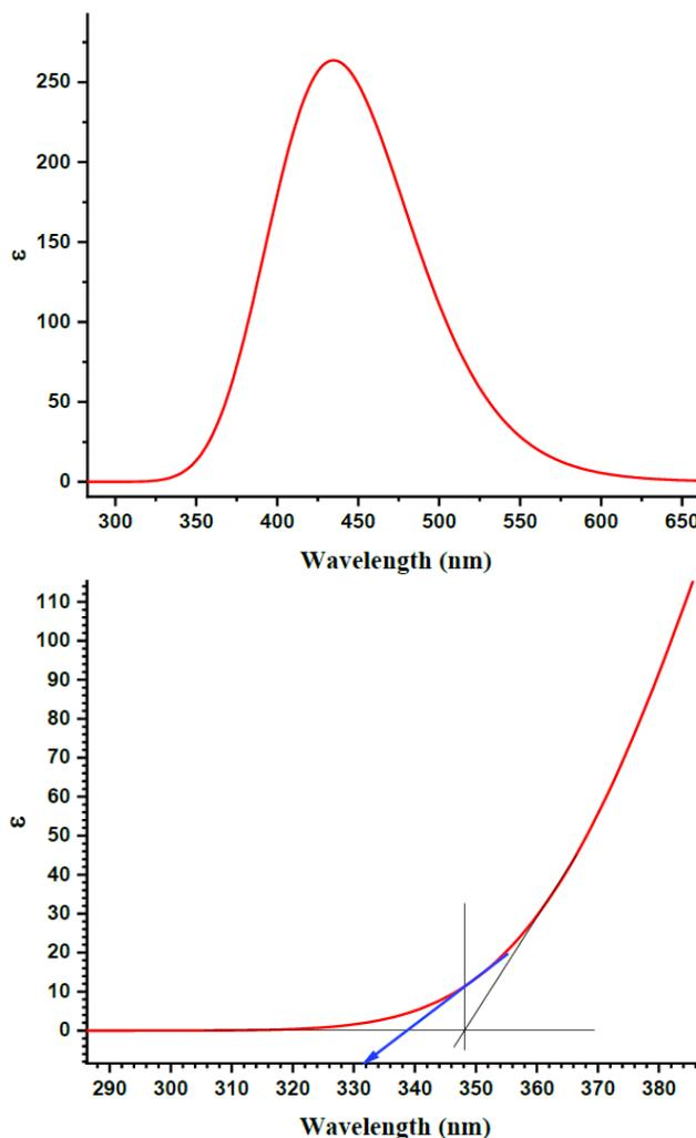
Fig. 6: (a) UV-vis absorption spectrum and (b) edge wavelength of silicon hydride nanocluster.
