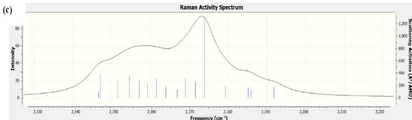
Fig. 4: (a) Raman spectrum of silicon hydride nanocluster, (b) inset of the spectrum in far and mid infra-red region, and (c) inset of the spectrum in mid infra-red region
