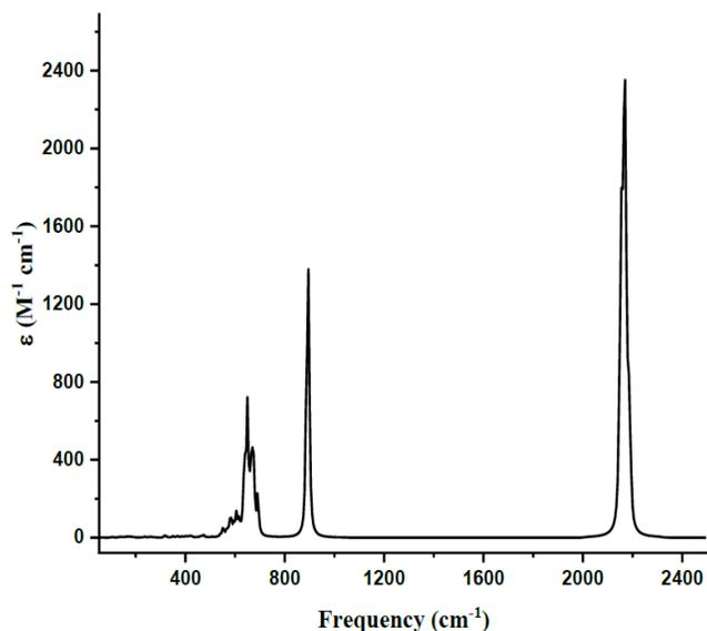
Fig. 5: IR spectrum of Silicon Hydride
