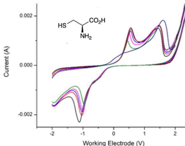
**Figure 1:** Cyclic voltammograms for increasing concentration of L-cysteine at phosphate buffer pH 8 and scan rate  $50 \text{ V/s}$
