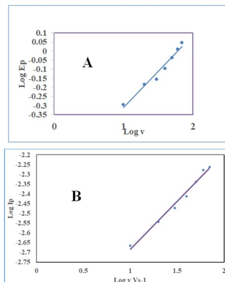
**Figure 4:** (A) Dependence of oxidation peak potential of cysteine on the square root of scan rate. (B) Linear relation between logarithm of peak current and logarithm of scan rate
