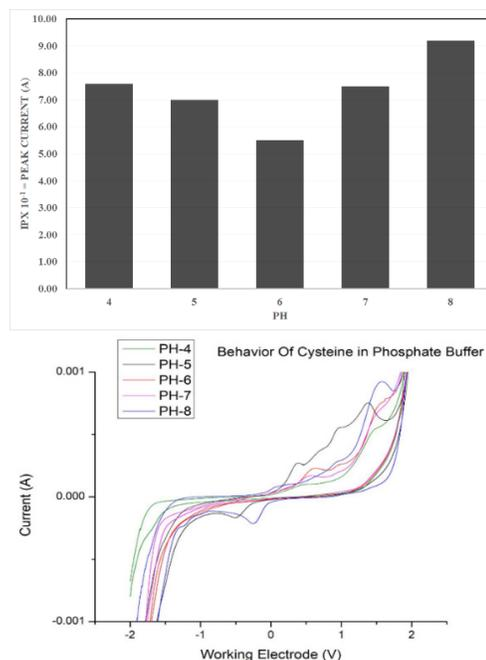
**Figure 2:** Cyclic voltammograms showing the effect of electrolyte and pH on cysteine oxidation. Phosphate buffer at pH 4.0 to 9.0 provides the highest peak current and stability
