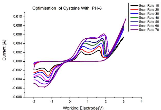
**Figure 3:** The cyclic voltammograms of the electrochemical oxidation of cysteine in phosphate buffer (pH 8.0) at different scan rates (10–70 mV/s)
