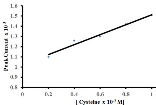
**Figure 5:** Calibration plot of peak current versus varying concentrations of L-cysteine, obtained by cyclic voltammetry at pH 8.0
