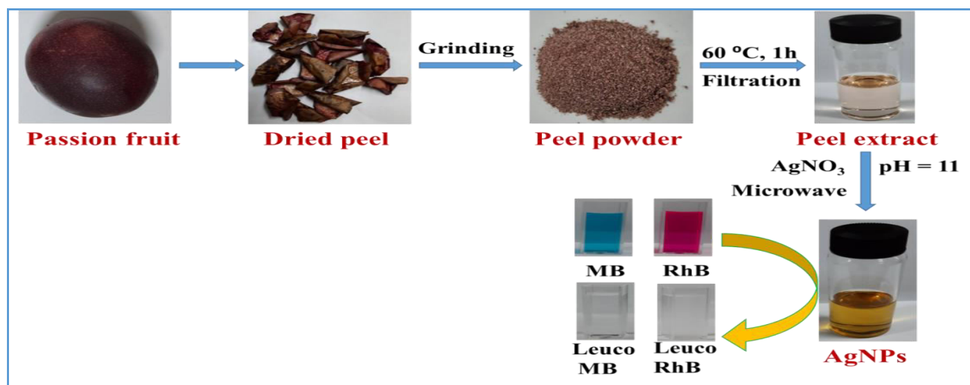
Scheme 1: Flowchart of preparation of PF capped AgNPs and its application for catalytic activity.
