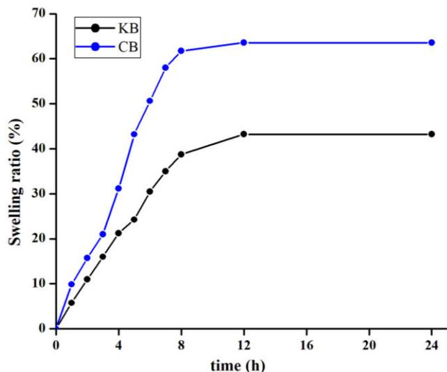
Fig. 4: Swelling behaviour of bead capsules as a function of time for formulations with Encapsulated Karanj oil emulsion beads (KB) and Encapsulated Castor oil emulsion beads (CB)
