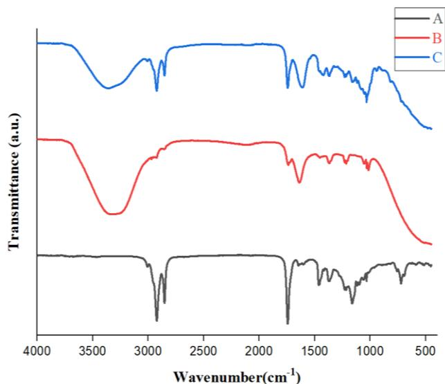
**Fig. 1: FTIR spectra of A) Karanj oil, B) Karanj oil emulsion and C) Encapsulated Karanj oil emulsion bead**
