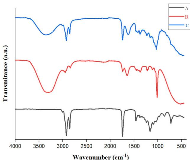
**Fig. 2: FTIR spectra of A) Castor oil, B) Castor oil emulsion and C) Encapsulated Castor oil emulsion bead**
