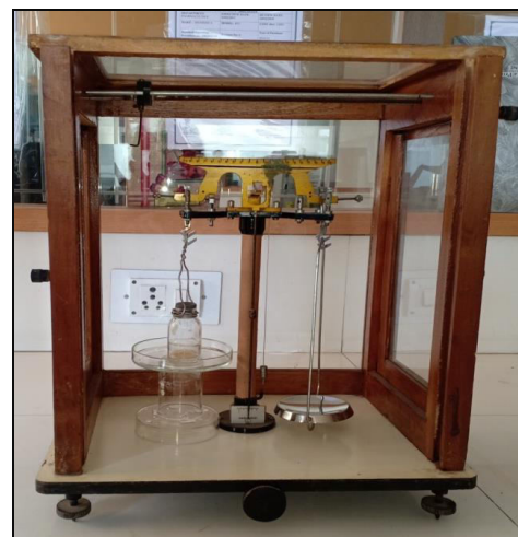
Fig. 1: Modified Muco-adhesive Tester
