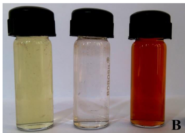
Fig. 1B: Leaves extract, Silver nitrate (1mM) and Reaction mixture (9:1) respectively from left to right
