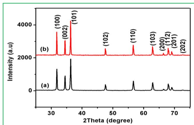
**Fig. 1: XRD spectra of synthesized ZnO (a) and Mg-ZnO (b) NPs for average crystalline size**
