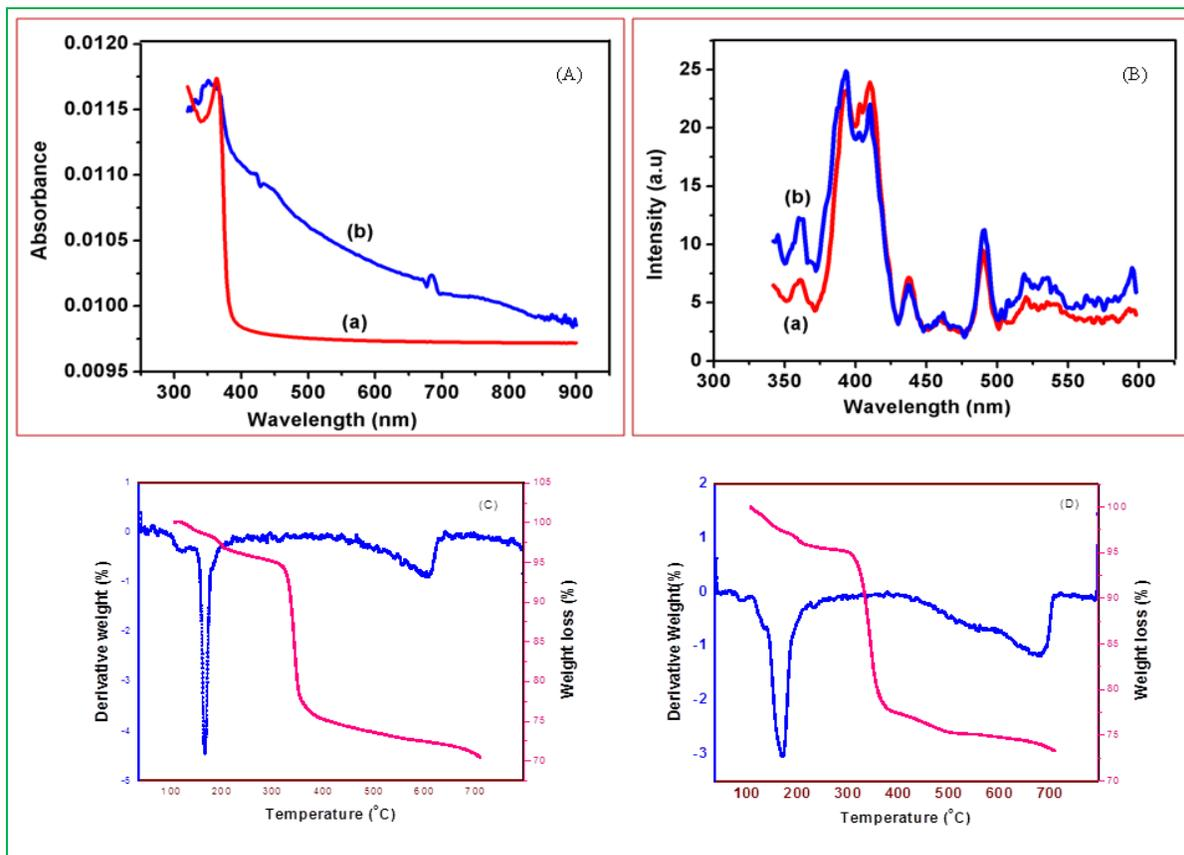
**Fig. 2: Optical (A) spectra, PL (B) of synthesized ZnO (a) and Mg-ZnO (b) NPs and DTA/TGA of (C) ZnO and (D) Mg-ZnO NPs.**
