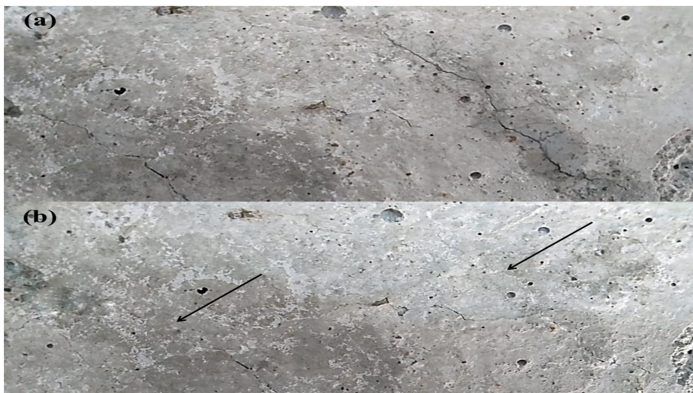
Fig. 5: Remediation of concrete cracks in the cement mortars. (a) mortar cracks seen on 0 day (before treatment); (b) calcite filled cracks indicated by solid arrows 14 days post-injections with cementation solution containing Bacillus cereus SSS1 bacterial suspension
