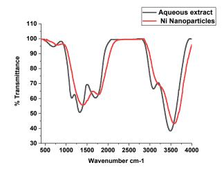
Fig. 2: FTIR spectra of *T. Chebula* fruit extract and Ni NPs
