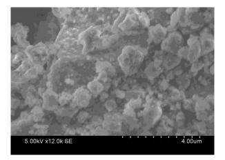
Fig. 4: SEM images of Ni NPs
