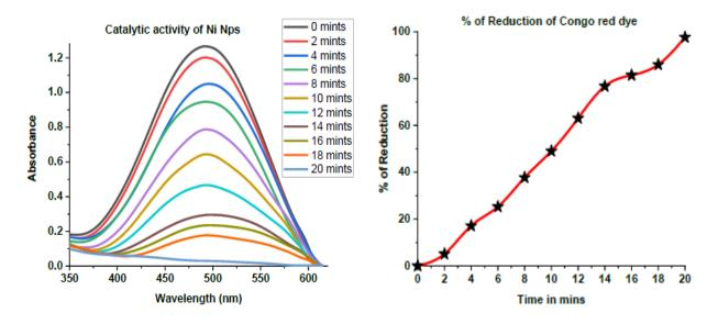
Fig. 7: a) Plot of catalytic activity of Ni NPs, b) % of reduction of CR by Ni NPs
