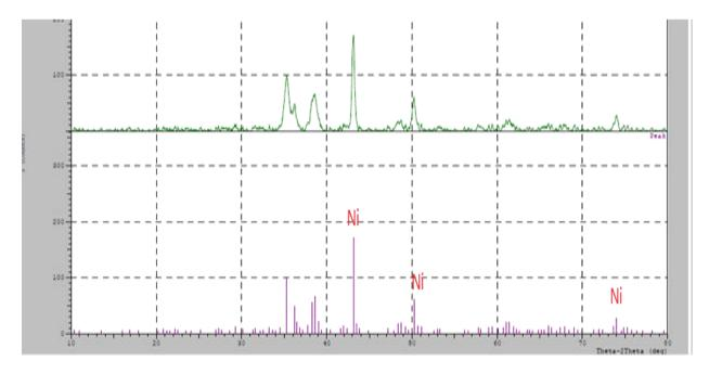
Fig. 3: XRD patterns of bio-synthesized Ni NPs sample
