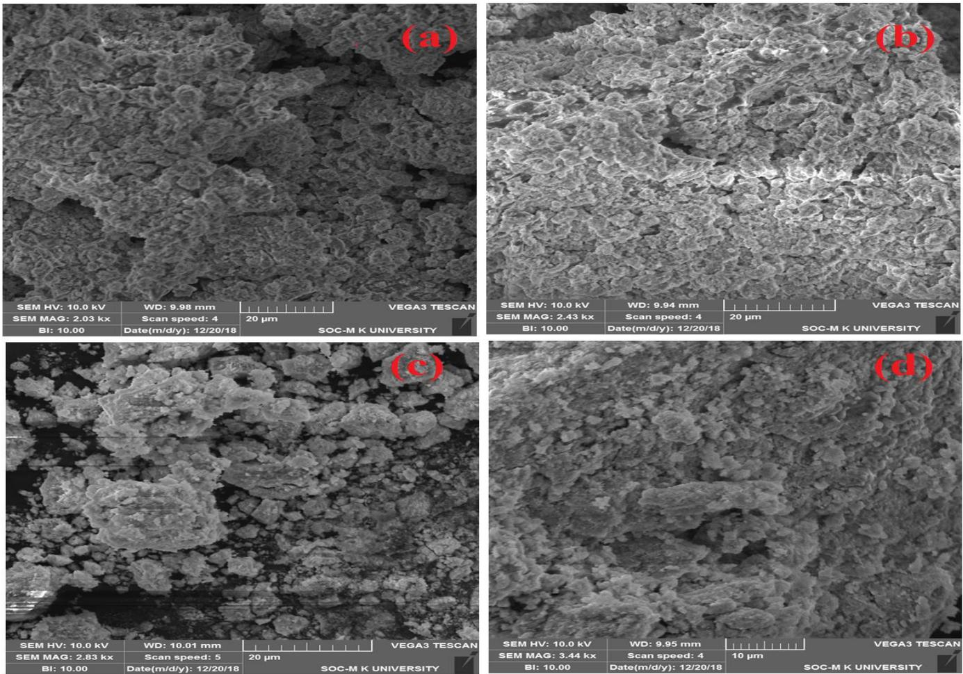
Fig.2: SEM images of bare ZnO-In<sub>2</sub>O<sub>3</sub> (a, b) and Au-ZnO-In<sub>2</sub>O<sub>3</sub>-Pt nanocomposites (c, d)
