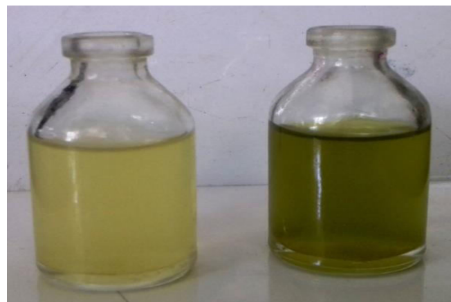
Fig. 8: The colorimetric colour change of ligand and ligand+ \text{Cu}^{2+} ion.
