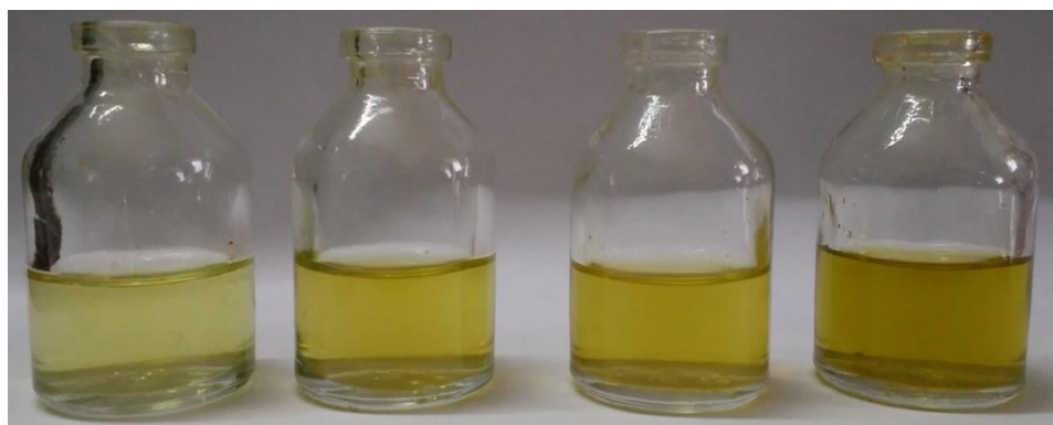
Fig. 9: The colorimetric colour change of ligand on addition of \text{Cu}^{2+} ion (first one from left side only ligand and 5, 10, 20 and 40 ppm \text{Cu}^{2+} with ligand)
