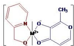
Fig.2: Tentative structure of ternary complex having HMP, M^{2+} and MA
