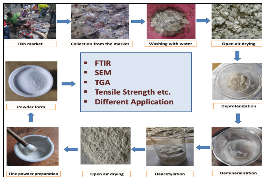
Fig. 2: Method of extraction of chitin and preparation of chitosan from fish scales
