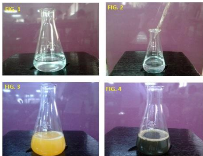
Fig. 1: \text{CuSO}_4 \cdot 5\text{H}_2\text{O} dissolved in D/W, Fig. 2: PEG 6000 was added to the aqueous solution, Fig. 3: Ascorbic acid and NaOH was added to the synthesis solution, Fig. 4: \text{NaBH}_4 was added to the solution. An instant color change occurred from yellow to black which indicated the presence of CuNPs
