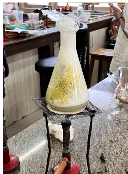
Fig 4: bleaching treatment with hydrogen peroxide
