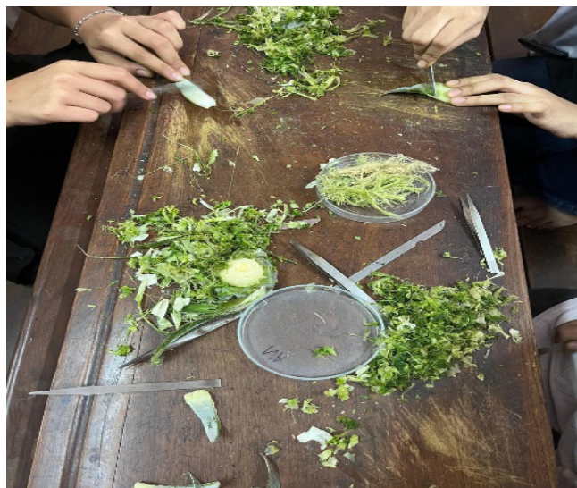
Fig. 2: Mechanical scraping of pineapple fibers from the leaves using a scalpel
