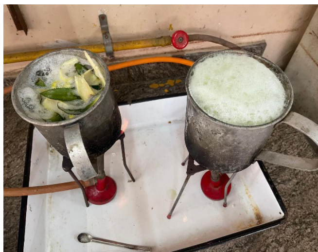
Fig 3: alkali treatment with sodium hydroxide
