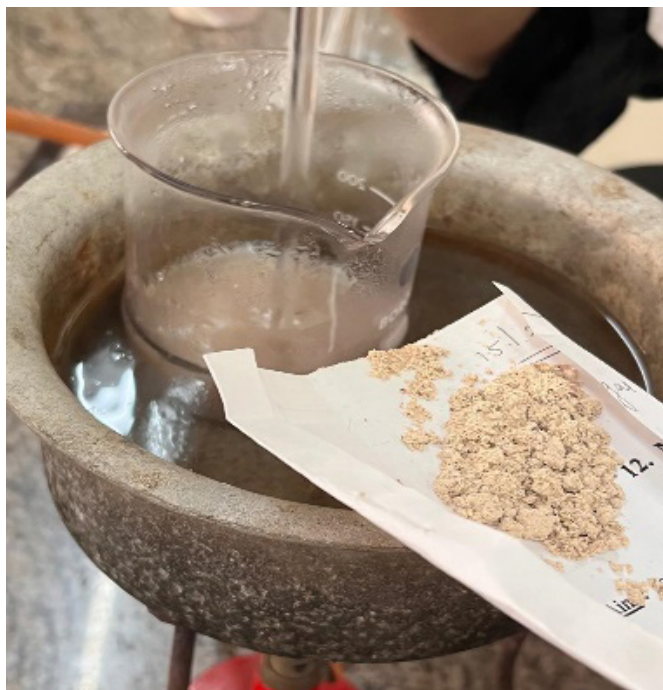
Fig. 5: Preparation of tamarind seed Polysaccharide (TSP) solution
