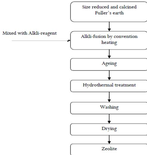
Fig. 1: A General flow diagram for the Synthesis of Zeolite by conventional method
