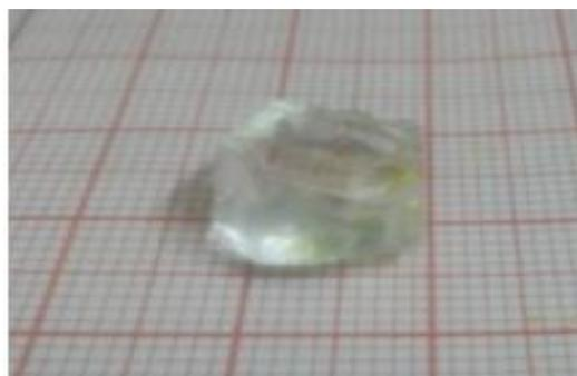
**Fig.1: The photograph of grown LLOA crystal**
