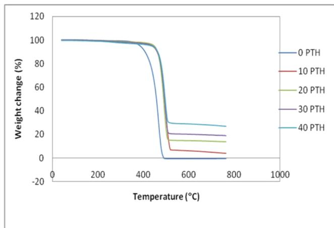
**Fig. 9: Thermogravimetric curves of PP and PTH/PP composites**
