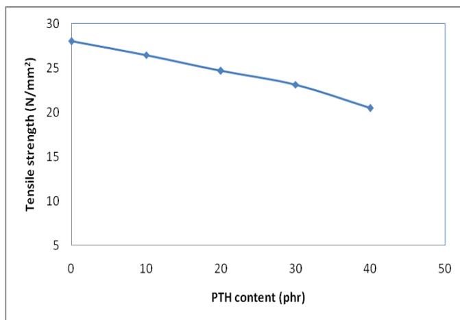
**Fig. 6: Variation of tensile strength with PTH content in PTH/PP composites**
