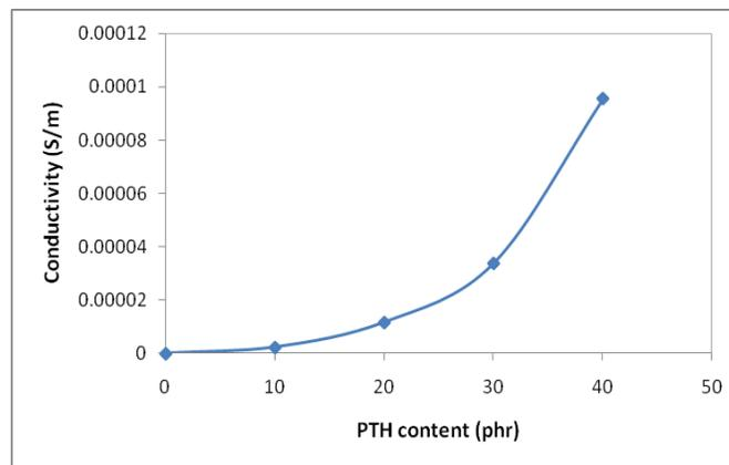
**Fig. 11: Variation of conductivity with PTH content of PTH/PP composites**
