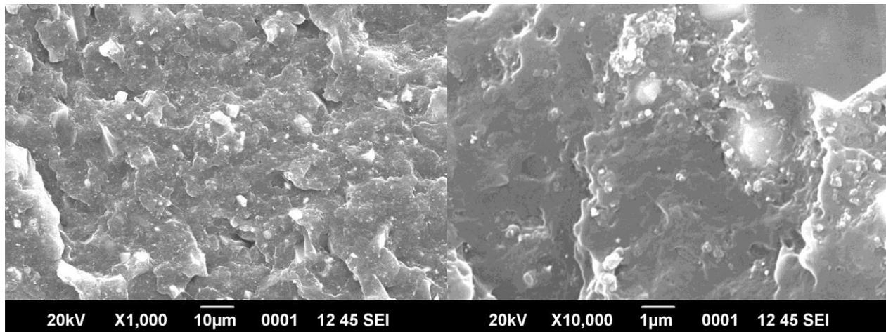
**Fig. 5: SEM image of PTH/PP composite**
