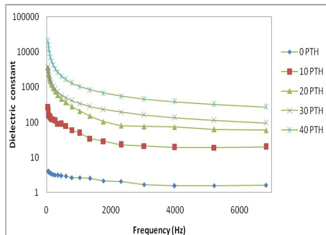
**Fig. 15: Variation of dielectric constant of PTH/PP composites with frequency**
