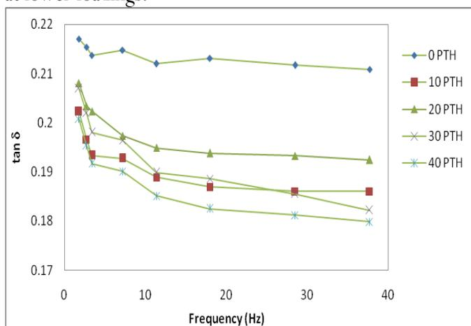
**Fig. 14: Variation of  $\tan \delta$  of PTH/PP composites with frequency**
