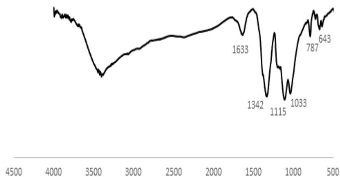
**Fig. 2: FTIR spectrum of prepared polythiophene**
