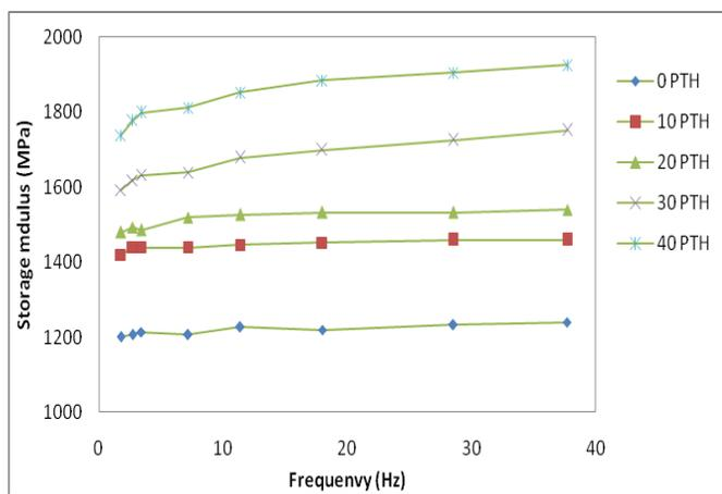
**Fig. 12: Variation of storage modulus of PTH/PP composites with frequency**
