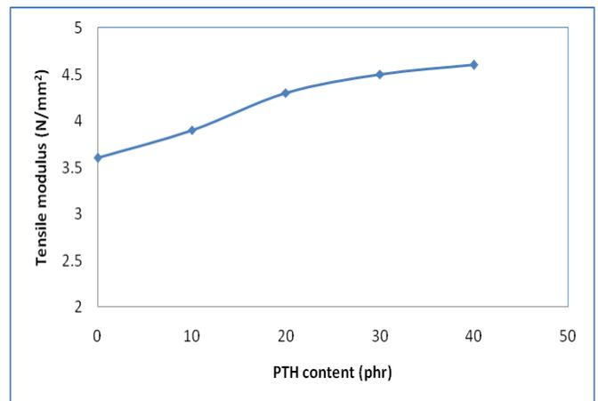
**Fig. 7: Variation of modulus with PTH content in PTH/PP composites**
