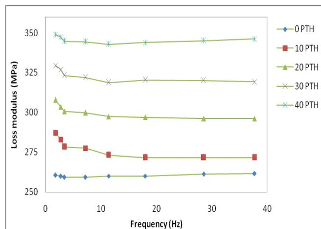
**Fig. 13: Variation of loss modulus of PTH/PP composites with frequency**
