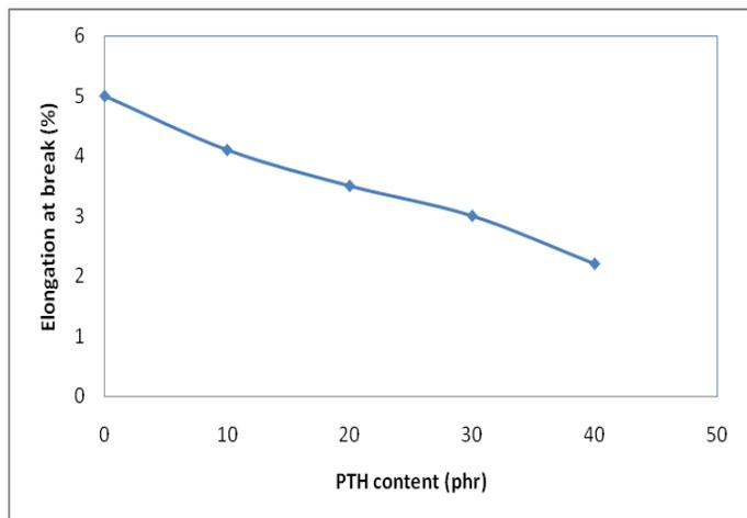
**Fig. 8: Variation of elongation at break with PTH content in PTH/PP composites**
