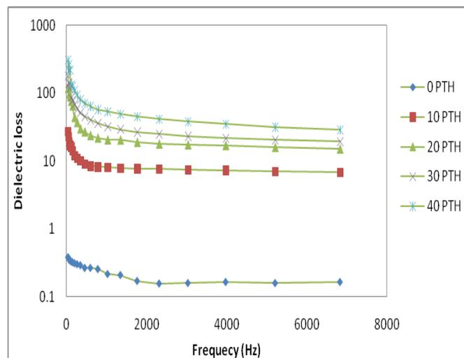
**Fig. 16: Variation of dielectric loss of PTH/PP composites with frequency**
