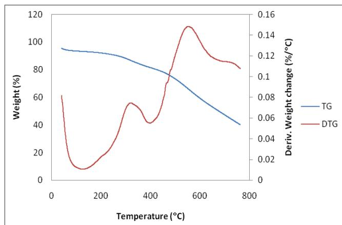
Fig. 4: Thermogravimetric and derivative thermogravimetric curves of PTH
