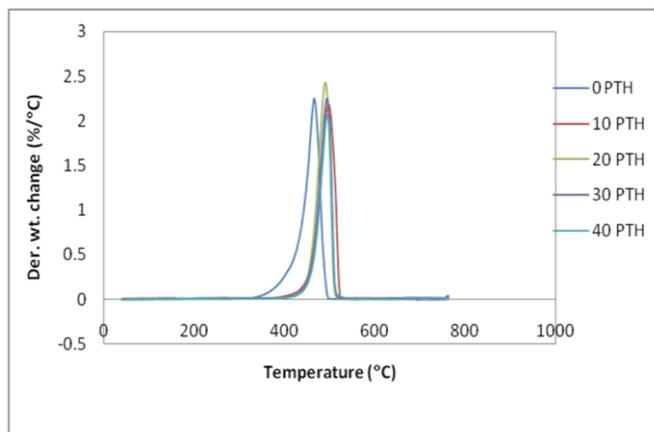
**Fig. 10: Derivative thermogravimetric curves of PP and PTH/PP composites**
