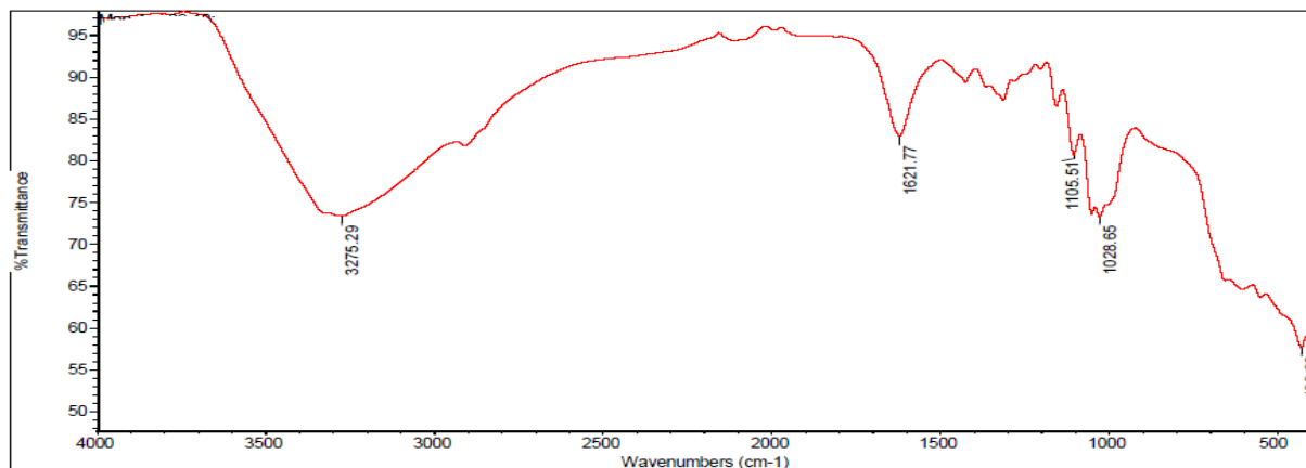
Fig.5: (b) FTIR Spectrum of Carbon steel in JGL extract in 1.0N HCl
