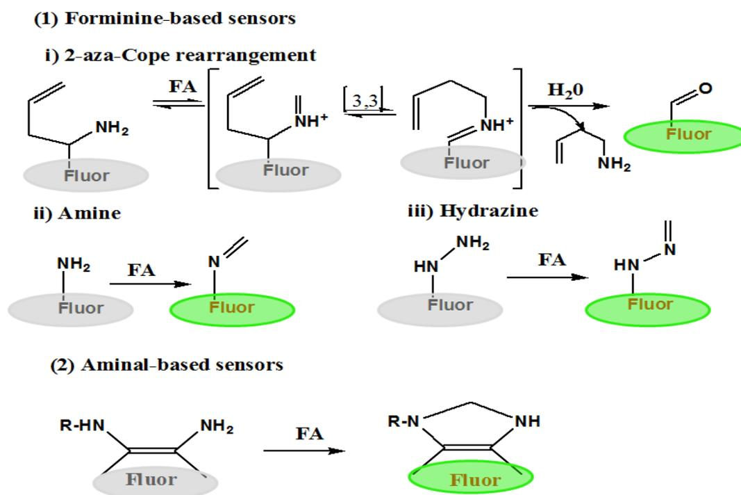
Fig. 1: Different reactive sites of fluorescent probes and sensing mechanism for FA
