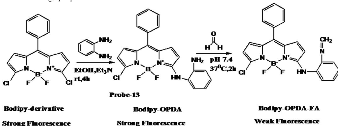
**Fig. 14: Design and sensing mechanism of the probe-13**
