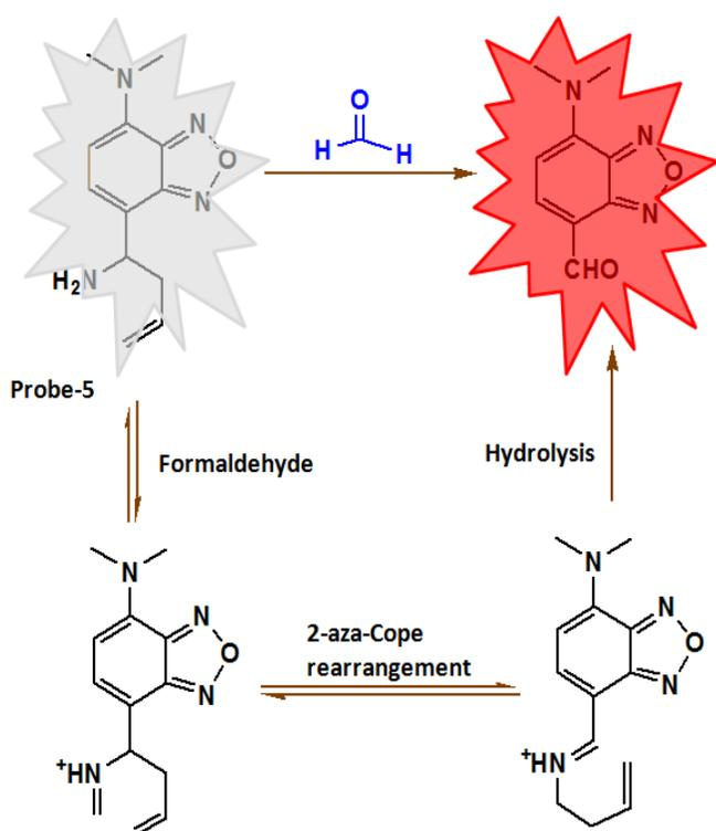
Fig. 6: Design and mechanism of the fluorescent probe-5
