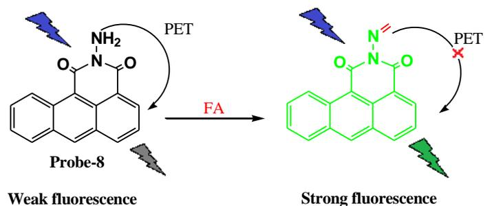
**Fig. 9: The proposed sensing mechanism of the probe-8 for FA**
