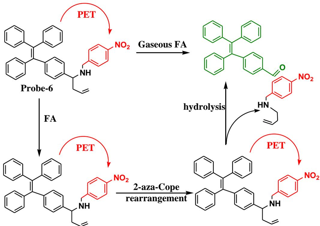
**Fig. 7: Schematic diagram and FA sensing mechanism of the probe-6**
