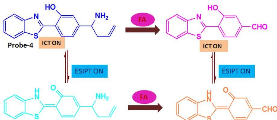
Fig. 5: Schematic diagram for FA sensing of the fluorescent probe-4
