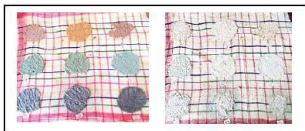
Fig. 6: handsheets prepared from bus tickets pulp a) just after treatment, b) After air-drying for 48 hours. control (left), P-C (middle), P-L (right)
