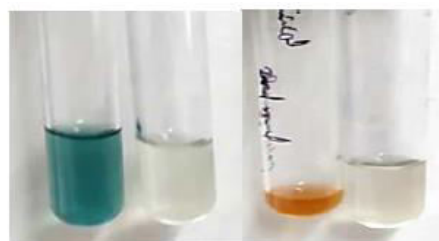
Fig. 2: Qualitative testing with a. 2mM ABTS and b. 10mM guaiacol for laccase obtained from P. ostreatus
