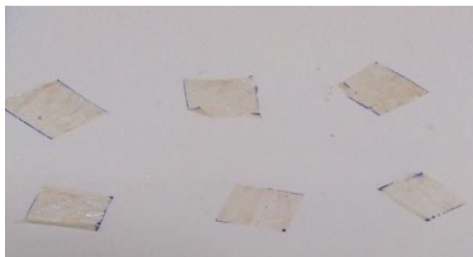
Fig.7: Degraded plastic sheets
