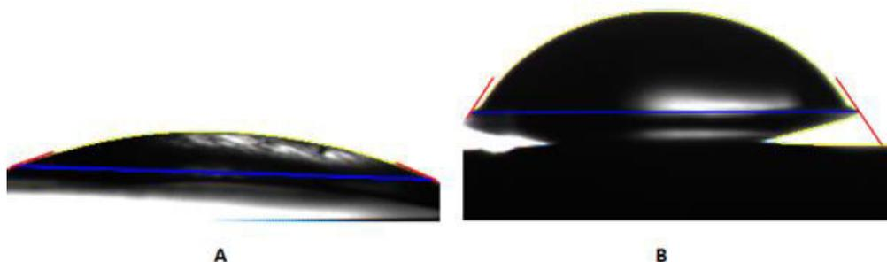
**Fig. 5: Contact angle of the synthesized CS (A) film and the CS-Ag nano hydrogel from *S. viminalis* (B)**
