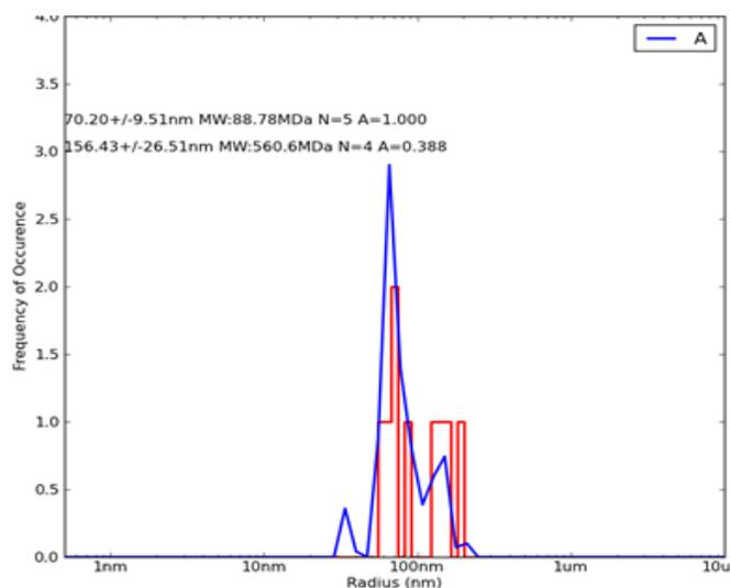
**Fig. 3: Particle size distribution curve for green synthesized silver nanoparticles from *S. viminalis***
