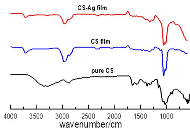
**Fig. 6: FTIR spectra of pure CS, CS hydrogel, and CS-Ag nano hydrogel from *S. viminalis*.**
