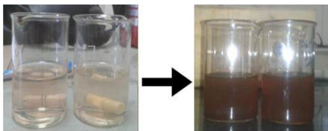
**Fig. 1: Green synthesis of Ag nanoparticles from *S. viminalis*: visible observation by changing the color from transparent to brown (from left to right)**
