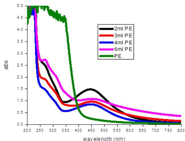
**Fig. 2: UV-visible spectra of silver nanoparticles from *S. viminalis*, reaction conditions with constant AgNO<sub>3</sub> (10 ml) and constant CTAB (1 ml) with different amounts of plant extract (PE)**
