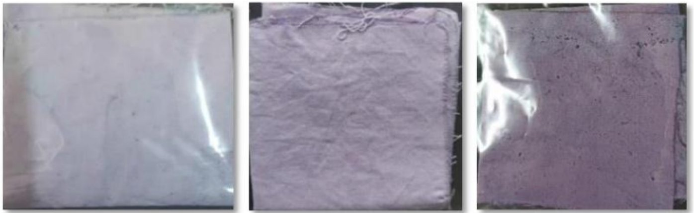
4a: Laundering using hot water 4b: Laundering using cold water 4c: Exposure to sunlight
