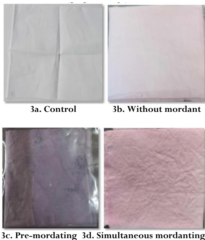
Fig. 3: Dyeing of Brassica oleracea L.(purple cabbage) waste extract on cotton fabric
