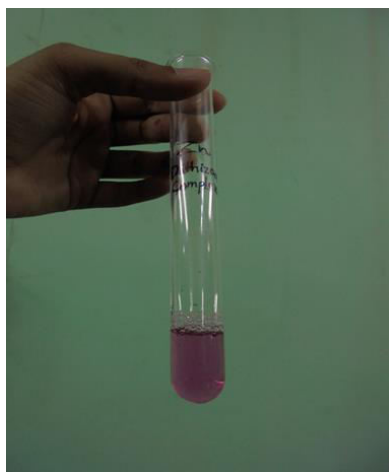
Fig. 14: Pink coloured Zn 2+ -Dithizone complex after Dithizone reaction for Zn 2+
