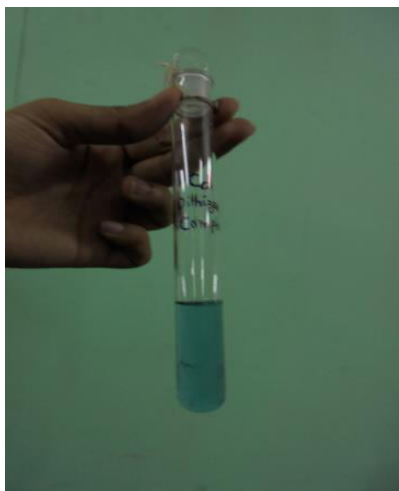
Fig. 15: Green coloured Cd 2+ -Dithizone complex after Dithizone reaction with Cd 2+
