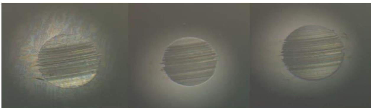
Fig. 7: Microscopic image of Wear scar diameter - 2% short chain alkyl DTP compound in Mineral oil
